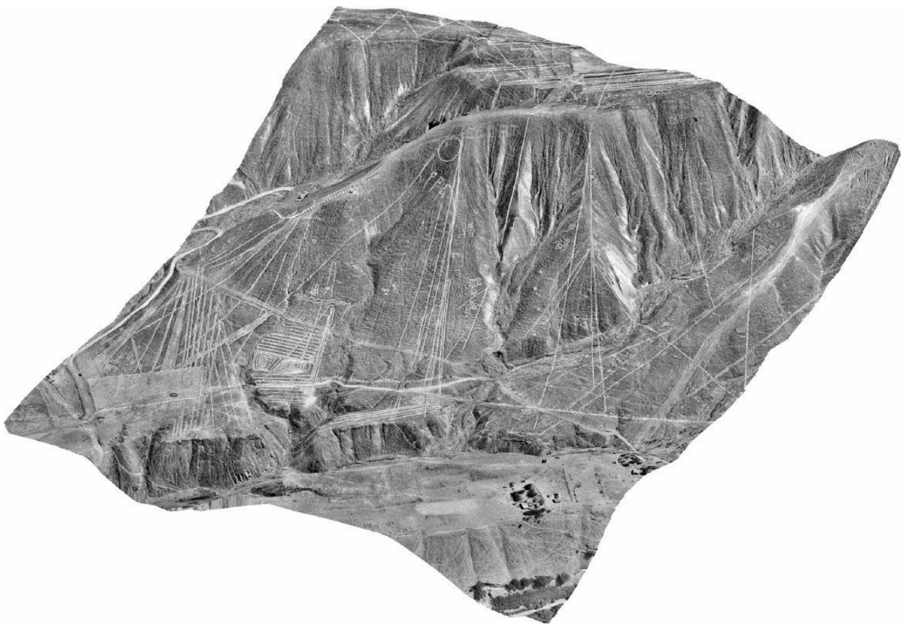
Fig. 7: Synthetic 3-D view (DTM with orthoimage texture and vector overlay) of site PAP 50 with spirals, lines and anthropomorphic figures
